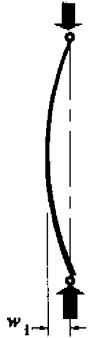
Figure E.2: Initially crooked bar.
